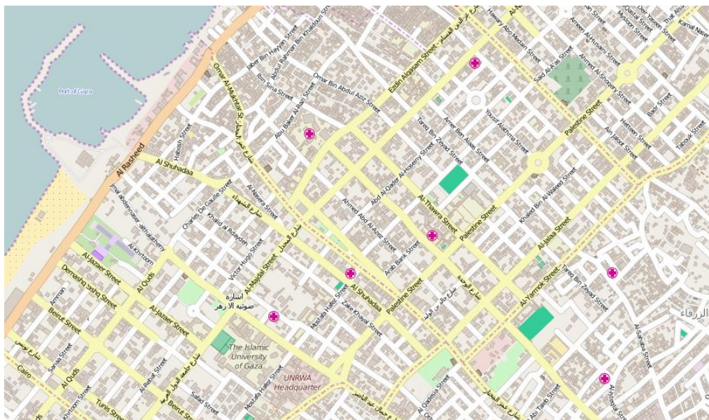
Figure (3.2): Street and parcels orientations in Gaza Strip, (open street map, 2015) (Street and parcels take parallel and perpendicular orientations to the sea coast in Gaza Strip.)
